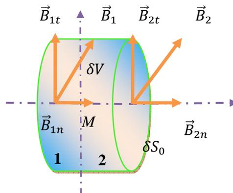
$$\iiint_{\delta V} \vec{\nabla} \cdot \vec{B} \, d\tau = 0 = \oiint_{\delta S} \vec{B} \cdot \vec{dS} = (B_{2n} - B_{1n}) \delta S_0$$
